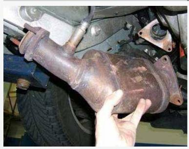
Remove the nuts that connect the catalytic converters to the exhaust manifolds, and then remove the converters from the vehicle.
